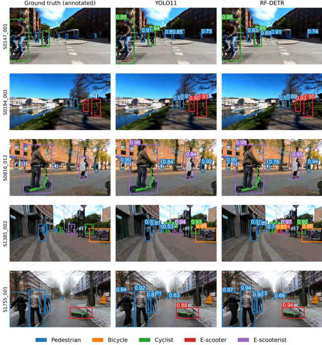
Figure 5: Successful example predictions on images from unseen test-set scenes for YOLO11 and RF-DETR, shown alongside ground-truth annotations. Numbers indicate predicted confidence scores (threshold = 0.5).
