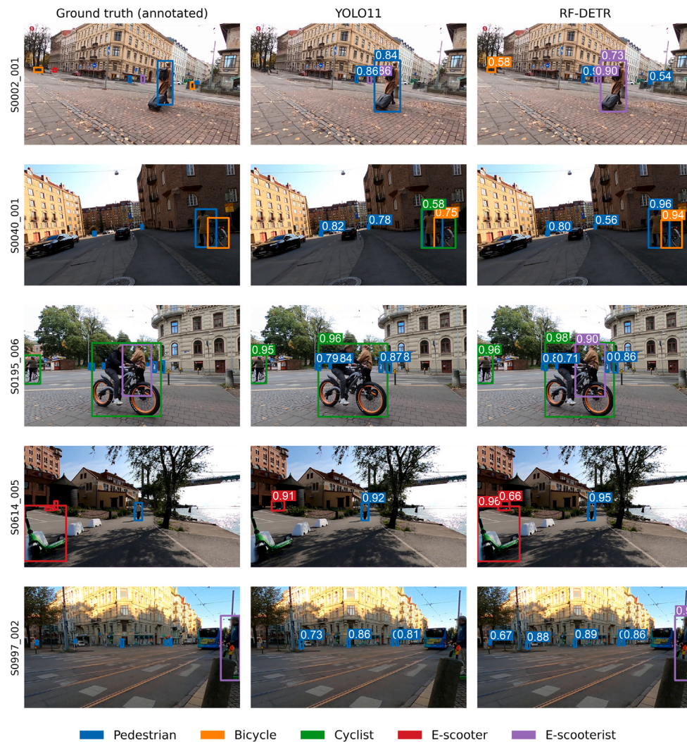
Fig. 6. Representative examples of prediction errors from YOLO11 and RF-DETR, shown alongside ground-truth annotations.
