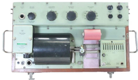
Figure 8. Level recorder Type 2301, source: archive Applied Acoustics.
