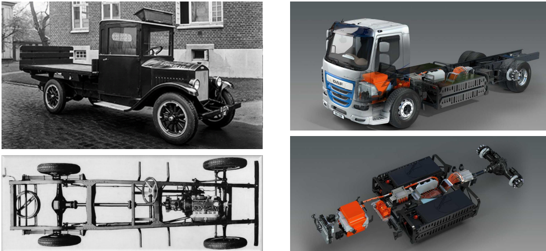
Figure 1.1: Illustration of a 4x2 vehicle configuration, with chassis mounted prime mover and rear axle drive; (left): Historical diesel engine layout on Volvo ÖV4 TV pickup vehicle from 1927 [110]. (right): DAF LF Battery Electric Innovation Truck exhibited at IAA 2018 [35].
