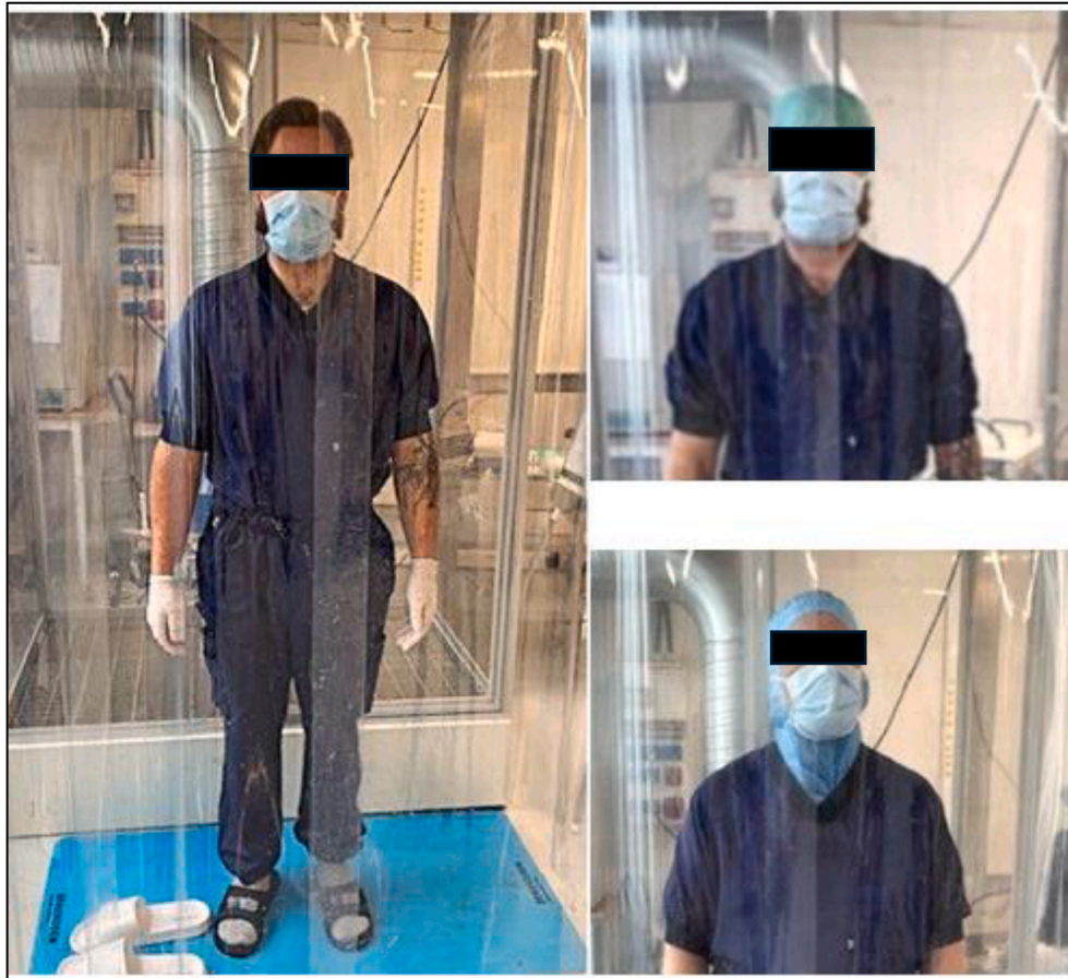
Figure 2. A test person without headgear standing outside the test chamber (left), and to the test persons with a disposable cap (top right) and disposable hood (bottom right).
