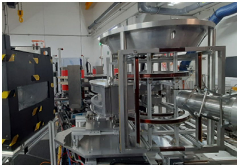
Fig. 16 The wide-angle polarization analyzer installed on Larmor, surrounded by a 3D coil set for XYZ polarization control. Photo: Oskar Štepančić
