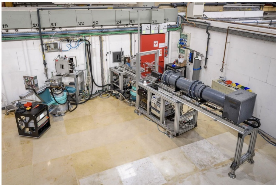
Fig. 1 Photograph of the Super-ADAM instrument at the Institut Laue-Langevin. The high flux and high resolution mode are visible on the left and right hand side, respectively
