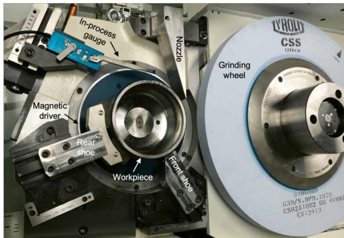
Fig. 2. Lidköping SGP 320 shoe-centerless grinding machine configured for high-volume external cylindrical grinding of bearing outer rings.
