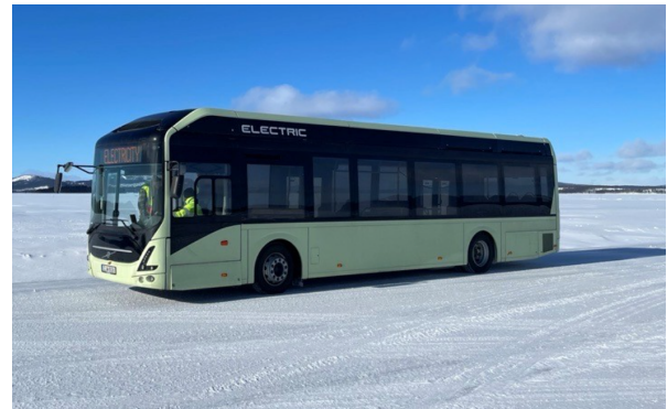
Fig. 1: Test Vehicle used for modeling, simulation and real tests: 4x2 battery-electric city bus
