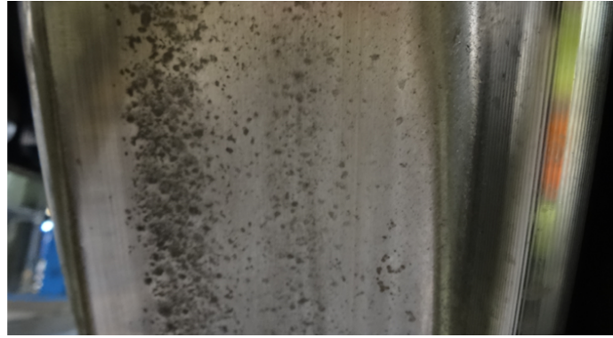
Figure 5: Indentations caused by gravel
