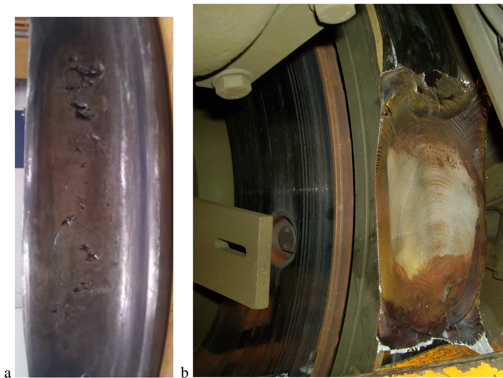
Figure 8: a) RCF cluster with material fall-out in a long segment, b) Subsurface initiated rolling contact fatigue fracture.
