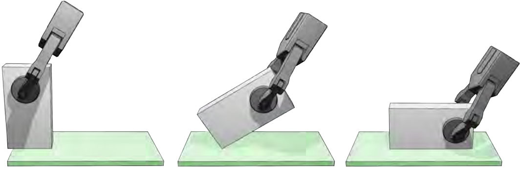
Figure 4.5: Illustration of hinge control while pivoting on an external surface.
