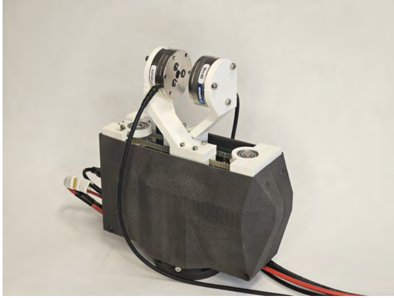
Figure 3.5: F/T sensors mounted on the fingers of gripper V1.
