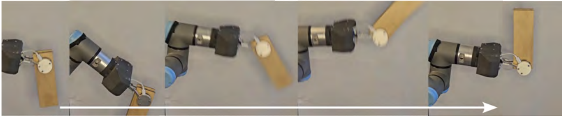
Figure 4.7: Time series of swing-up motion with hinge control.
