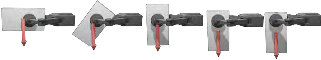
Figure 4.9: Illustration of the linear slip controller, starting with an initial torque that induces rotation followed by linear slip motion.
