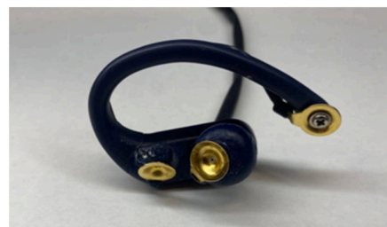
Figure 3. Ear-EEG signal acquisition device using gold electrodes.
