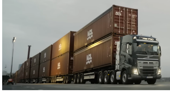
(b) A Volvo FH tractor towing 20 trailers and 750 tons [11].
