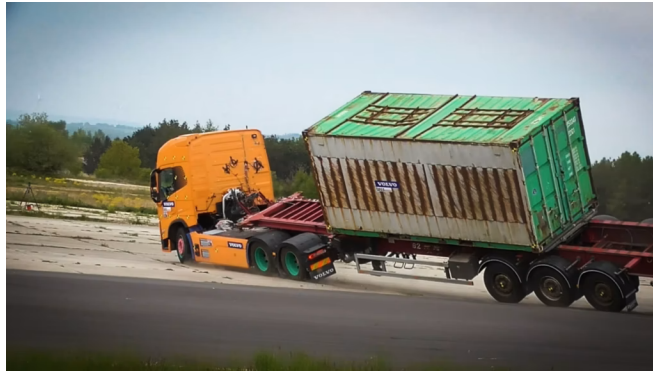
Figure 4.6: A tractor-semitrailer combination rolling over during electric truck crash safety tests [31].
