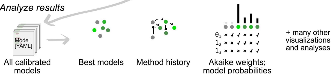
Fig 1. Model selection workflow with PETA Select. (1) The user defines the model selection problem , including the model space and the mathematical description of the set of possible process components, in the standard . (2) The user runs model selection via a calibration tool by sending the PETA Select problem to the PETA Select package , which initiates iterations of model selection. (2a) The package provides model candidates to the calibration tool based on the problem specification and the available calibration results. (2b) The calibration tool calibrates the proposed candidate models and sends the calibration results to the package. Iterations of (2a) and (2b) continue until the package sends a termination signal to indicate the end of model selection. The results are provided in the PETA Select model format and include all calibrated models with their calibration results. (3) The package can be used to perform subsequent analyses and visualizations of the results.
