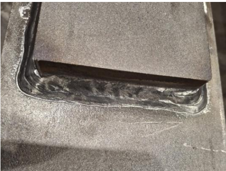
Figure 2 HFMI treatment of cover plate ends.
