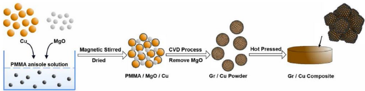
Figure 3.5: Schematic representation of the in-situ growth of graphene on Cu powder using PMMA as a carbon source and MgO as a dispersant. Reprint from Wang et al. [97] under Creative Commons license .
