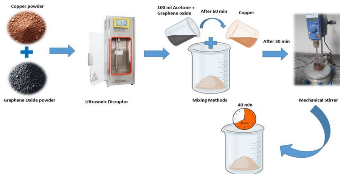
Figure 3.3: Schematic representation of the solution-assisted incorporation of GO into Cu powder using ultrasound followed by mechanical stirring. Reprint from Souza et al. [92] under Creative Commons license.
