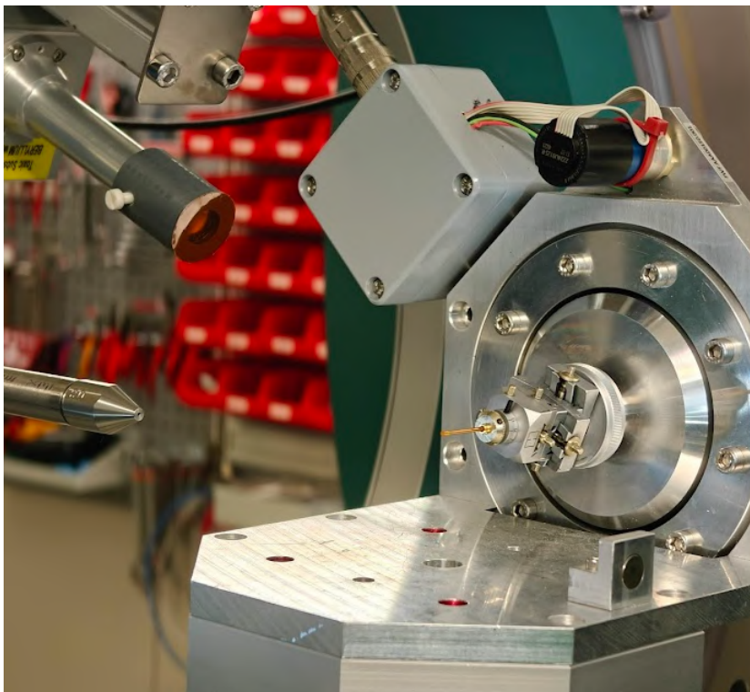
Figure 4.6: The XRD-1 diffractometer of the ROBL BM20 beamline (ESRF), showing the goniometer and capillary sample holder used for synchrotron measurements. Photo by the author.
