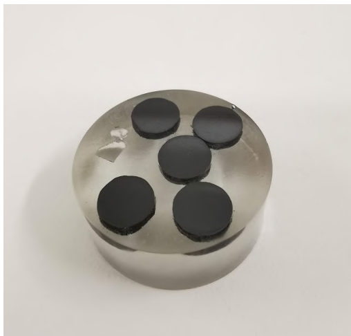
Figure 4.4: Lanthanide-doped \text{UO}_2 pellets mounted in epoxy prior to polishing and SEM microstructural analysis. Photo by the author.
