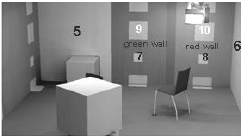
Figure 4. The areas in the lightest nuance were difficult to simulate. They appeared too greyish in the digital models. The small squares (7 and 8) that were strikingly whitish in reality were hardly noticed in the digital models. The light areas were painted in: 5 and 7: NCS S0510-G90Y; 6 and 8: NCS S0510-Y10R. The larger squares were painted in the stronger nuance of the yellow hues. On the red and green background area 9 (1030-G90Y) and 10 (1030-Y10R) appeared almost equal in hue.
