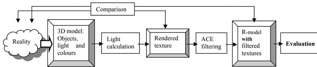
**Figure 3:** The ACE can be used for filtering rendered textures in a 3D model. These rendered textures are separate images of walls, floor and other surfaces in the room, used in Virtual Reality-models.
