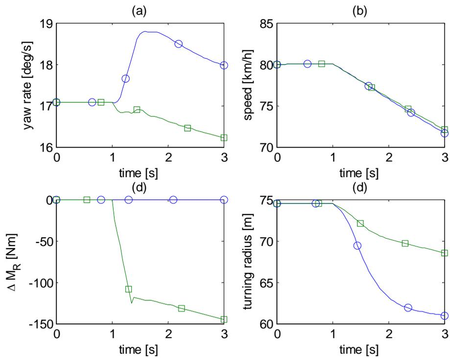
Figure 12: Yaw rate, speed and turning radius response under Drop Throttle In Turn (DTIT) maneuver under a fixed steering input ( $60^\circ$ ). The lines marked with a circle indicate a vehicle without eLSD and the line with square markers are a vehicle where the eLSD is locked when the throttle is dropped.
